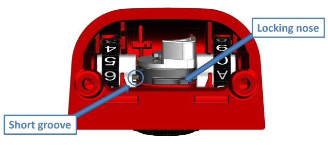
Turn the left-hand number wheel until the **short groove** of the number wheel is above the locking nose of the rotary knob
