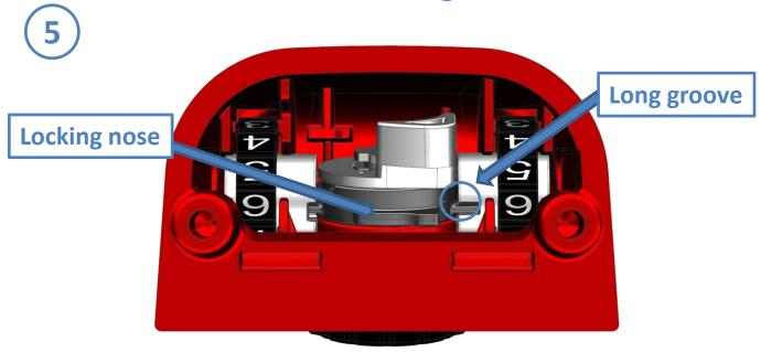
Turn the right-hand number wheel until the **long groove** of the number wheel is above the locking nose of the rotary knob
