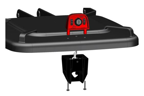
Open the lid and unscrew the upper lock part from below
